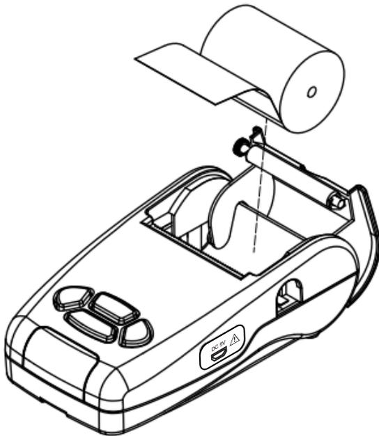
Lay the free end of paper over the printer head, past the serrated paper cutter onto the body of the front of the printer's case. Now close the paper cover and gently press down until it locks into place. Start the paper feed sequence to confirm that the paper has been correctly loaded. Tear off the excess paper by pulling it against the paper cutter.
