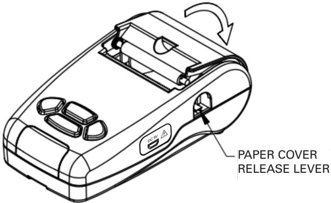
Remove the old paper roll core and insert the new roll so that it sits as follows :-
