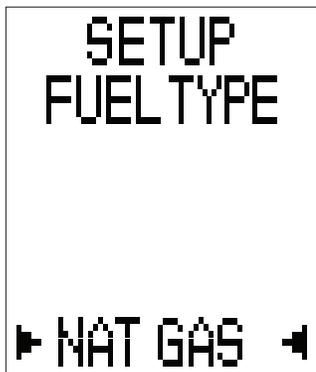
In Heat Exch Setup Screen, select Fuel type (Natural Gas, Propane, LPG, Light Oil, Heavy Oil, Bio Oil, Pellets, Butane)
