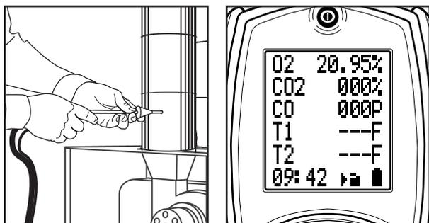
Remove the probe from the flue and allow analyzer to purge with fresh air until readings return to zero. O2 to 20.9%, CO to Zero (Be careful the probe tip will be HOT).
