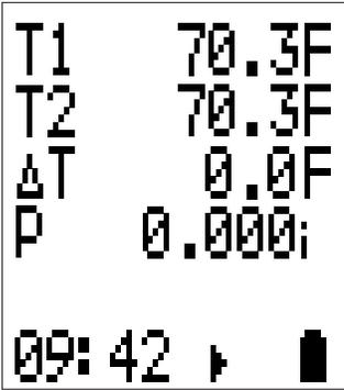
Use T1 connection for the Flue probe temperature sensor.
