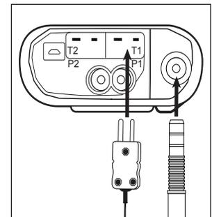
**NOTE:** Take care when inserting the temperature probes as the pins are polarized. Insert with the smaller pin (+) to the right.
