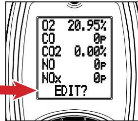
AUX displays 5 lines of editable parameters. To edit line values Press  $\blacktriangledown$  button until **Edit?** displays on the Status Bar.
