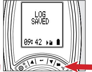
To Log: During testing, Press and Hold to log a report.
