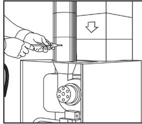
Insert flue probe into stack. Adjust cone so the probe tip is approximately at the center of the stack.
