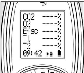
O2/Eff displays CO<sub>2</sub>, O<sub>2</sub>, Efficiency, Flue temperature, Inlet temperature.
