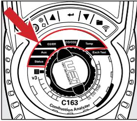
Rotate the dial to either STATUS, AUX, O2/Eff, CO/CO2 or Temp setting.
