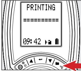
During testing, Press to start printing.
