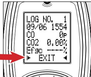
To EXIT, Press and buttons until EXIT is selected between two arrow icons. Press to EXIT screen.
