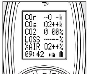
CO/CO<sub>2</sub> displays CO (ppm), CO<sub>2</sub>, Losses calculated, Excess air %. Make any adjustments needed for proper Combustion and wait for analyzer to display change in readings. (Repeat as necessary).
