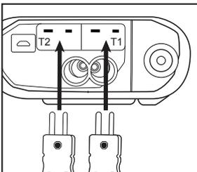
Insert K-type temperature probes into input T1 and T2.
