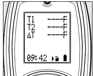
TEMP displays T1, T2 and Differential Temperature. (Pressure C163 C164 only)
