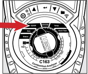
Rotate function rotary dial to O2/Eff for Test Screen 1 parameters.
